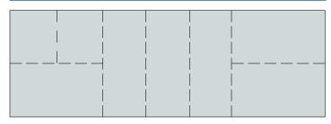
The sequential movement of SQUAREGAGE means different size blanks can be effectively sheared from a large blank to maximize material utilization.
