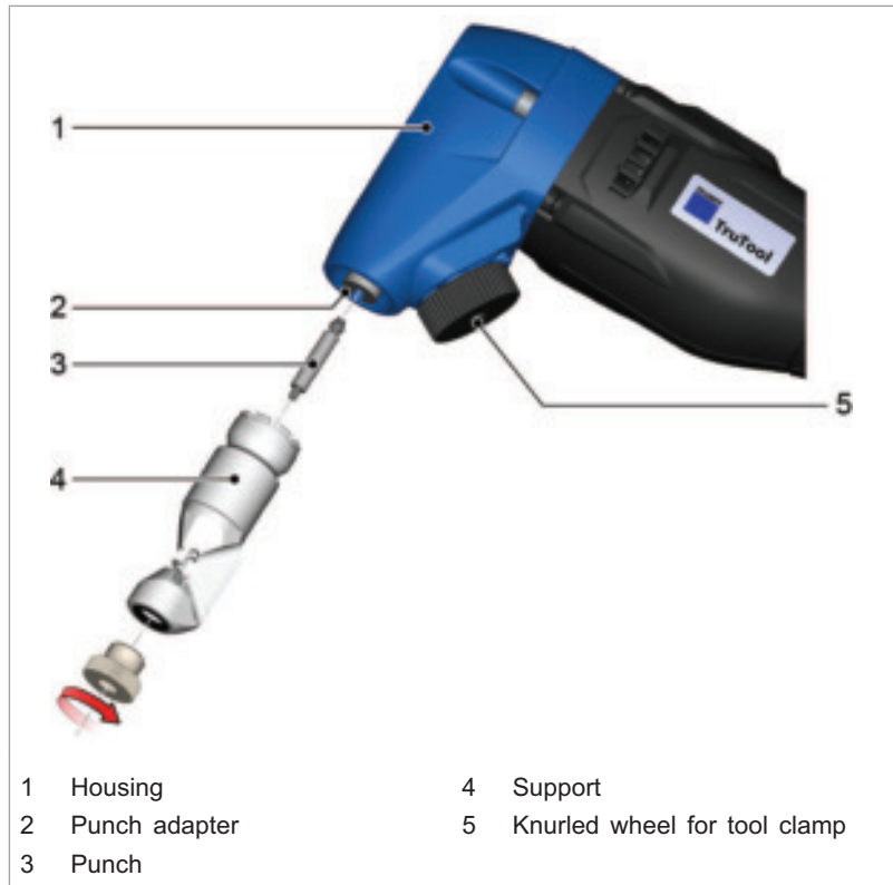
Replacing the tool
