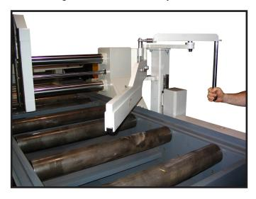
3. Rotate the bundling arm completely out of the loading area until the control link weldment seats on to the spool.
