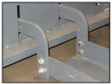
**7.** The barfeed coolant drain line is tied to the front leg. Cut and route through the cable trough into the chip tray of the saw. Be careful to not interfere with the travel of the chip paddle.
