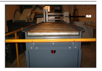
**17.** Fasten the shuttle datum side guard to the machine with the bolts provided.
