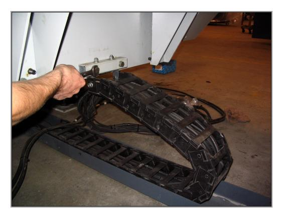
**9.** Remove the datum vise toggle cover - three 3/8 NC bolts on top, and two 3/8 NC bolts on the underside. Install the rod end of the cylinder with the 1/2 NF x 1.50 socket bolt. Fasten the lower cylinder eye with the 1/2 NC x 4.50 hex bolt. Zip tie the cylinder hoses (141 and 142) to the bottom of the carriage box centre. Re-install the datum vise toggle cover.
