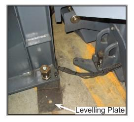
**3.** Connect the three lower struts that assemble the front leg of the barfeed to the saw. The finished gap between the front plate of the conveyor and the rear plate of the machine is to be 5/8" +/- 1/8". The alignment between the barfeed and machine should be checked quickly with a 10' piece of cold rolled flat bar or a laser. Adjust the struts if necessary.
