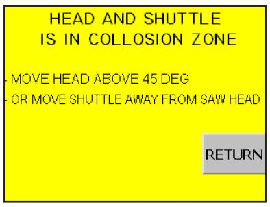
In such cases you will need to retract the shuttle to the back in order to clear the head to go to the required angle. In Manual Mode: It is a good idea to alter the cut if the required pieces involve this scenario. Flip the piece upside down and perform the cut when the head is turned 30 degrees towards the outfeed side of the machine where there is no possible collision as shown in the following example:
