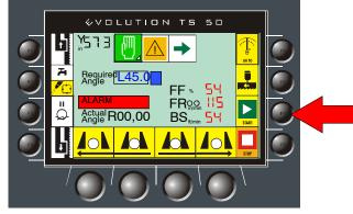
**N.B.** Tap on the touchscreen box shown in the figure to see problems during operation. The box will turn blue to indicate caution and red to indicate a machine alarm. See chapter 10 for a complete list of alarms.
