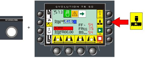
Press the button shown in the figure to start the cutting cycle holding the enable commands button pressed at the same time. The band will be start turning and the machine will start cutting.
