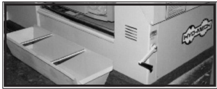
Manual chip conveyor handle and chip bucket.
