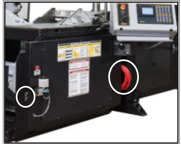
Coolant valve and wash hose
