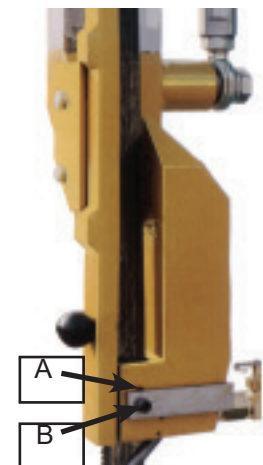
Blade guide adjusting screws.
