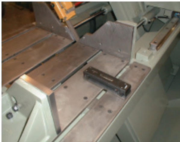
A machinists level being used in both directions
