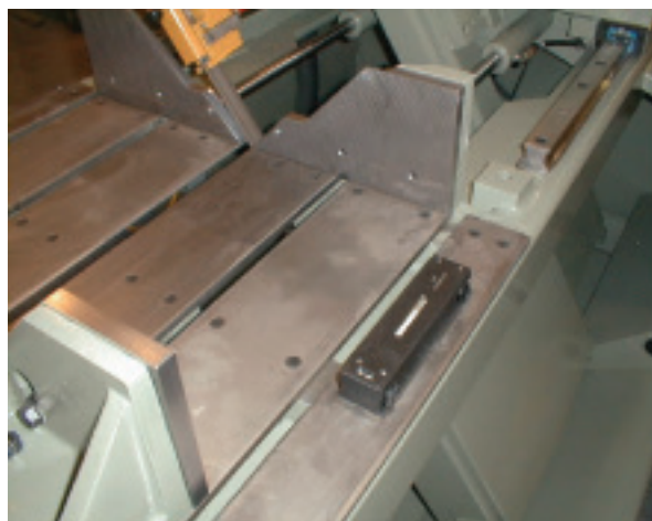
A machinists level being used in both directions
