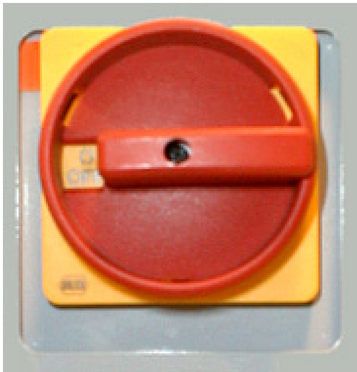
The main power disconnect switch used for safety lockout purposes.
