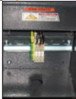
Power junction box without auto-transformer installed in the bandsaw. (240V & 480V) Drive Side of the Machine
