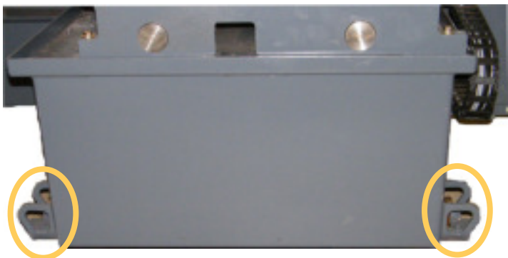
Levelling screw and anchoring hole on rear of the base
