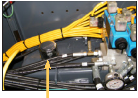
Oil Filler Cap found inside power pack door.
