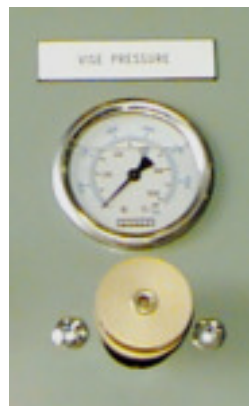
Variable Vise Pressure and Gauge
