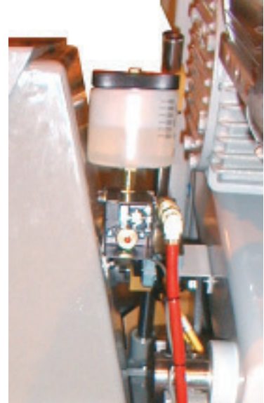
Flow adjustment dial for the mist lubrication system. Rated in drops per minute located behind the control panel.
