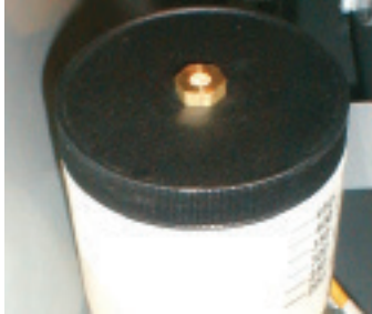
Air supply connection for the mist lubrication system located at the right side of the control console.
