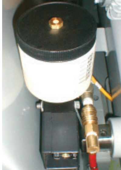
To turn the mist flow on, slide the valve forward and to turn it off, pull the valve back.
