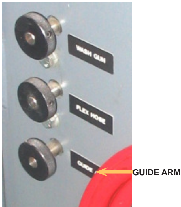
Coolant flow controls, found on left side of control console
