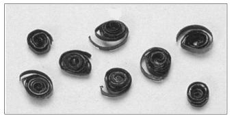
• Long coils of swarf indicate ideal cutting conditions.
