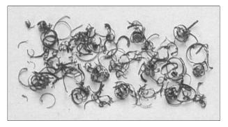
Thick and/or blue swarf indicates that the blade is overloaded.
