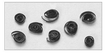
Long coils of swarf indicate ideal cutting conditions.
