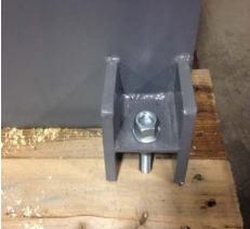
The base of the machine is anchored to the floor by two permanent studs located on the sides of the base. The studs are screwed into nuts previously sunk into the concrete, and tightened from above with lock nuts. The schematic specifications set out in Chapter 1 should be taken into account when positioning the machine.
