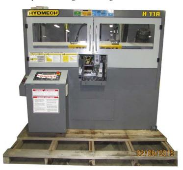
3. Remove the four lag bolts that hold the saw to the pallet (these will be used when anchoring the machine). The larger diameter hole is used for retaining during shipping and for use with concrete floor anchors. The smaller diameter, threaded holes are used for leveling the saw.
