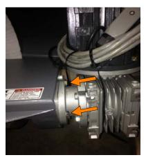
Auger assembly must be slid into machine and held in place by allen headed bolts provided.
