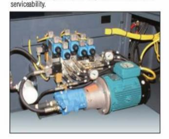
Hydraulic system controls all vising, head up/down, blade
